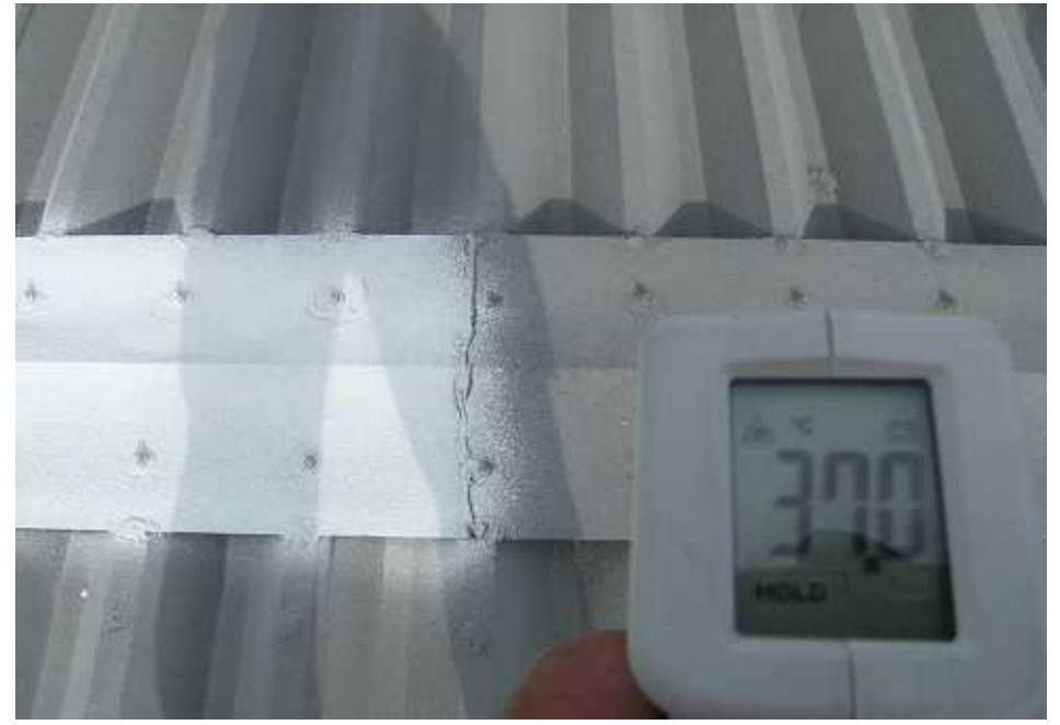
Temperature of Roof(Mighty coating only) 37 PM 16:00
